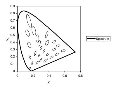
Figure 4 10-step MacAdam ellipses plotted on CIE 1931 chromaticity diagram
