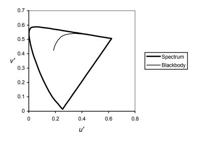
Figure 3 CIE 1976 uniform color space diagram
